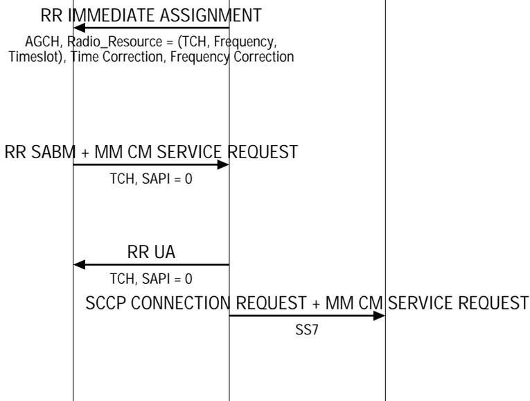
The BSS transmits the radio resource assignment to the Mobile via the AGCH channel. The message also contains the time and frequency corrections. The time corrections allow the mobile to time it's transmissions so that they reach the BSS only in the specified slot. The frequency corrections correct for the Doppler shift caused by the mobile's motion.
