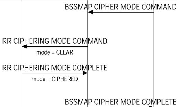
Since the subscriber has been successfully authenticated, the MSC initiates cipherng of the data being sent on the channel. The channel is cipherng so as so protect the call from eavesdropping.
