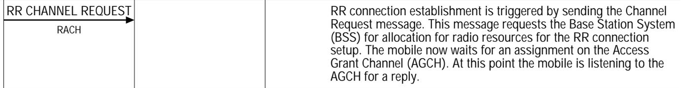
Note: The RR CHANNEL REQUEST is sent on a Random Access Channel (RACH). This is a slotted aloha channel that can be used at random, without any coordination between the mobiles. Any mobile can transmit on this channel whenever it wishes. If two mobiles transmit on the channel at the same time, their messages will be lost in a collision. The mobiles will detect the collision via a timeout and retransmit the message after a random back off.
