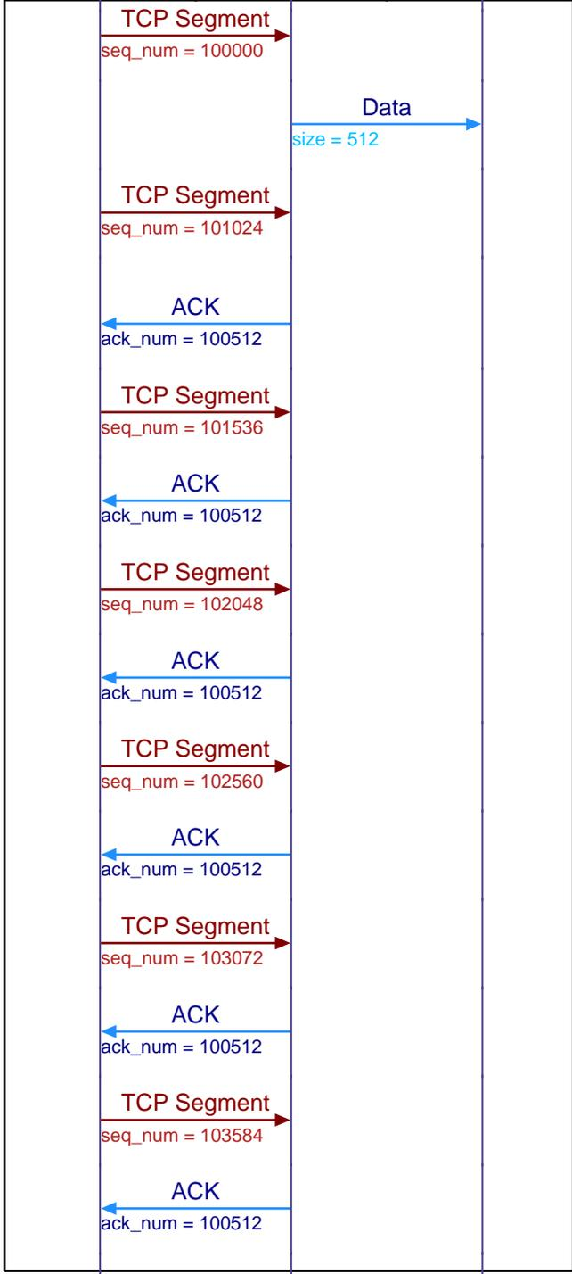
TCP segment (start sequence number = 100000) is delivered to the receiver
