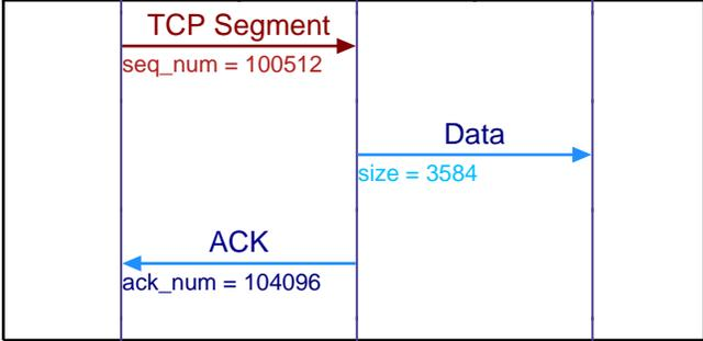
Finally, the retransmitted segment is delivered to the server
