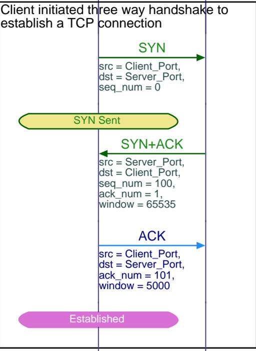
Client sets the SYN bit in the TCP header to request a TCP connection. The sequence number field is set to 0. Since the SYN bit is set, this sequence number is used as the initial sequence number
