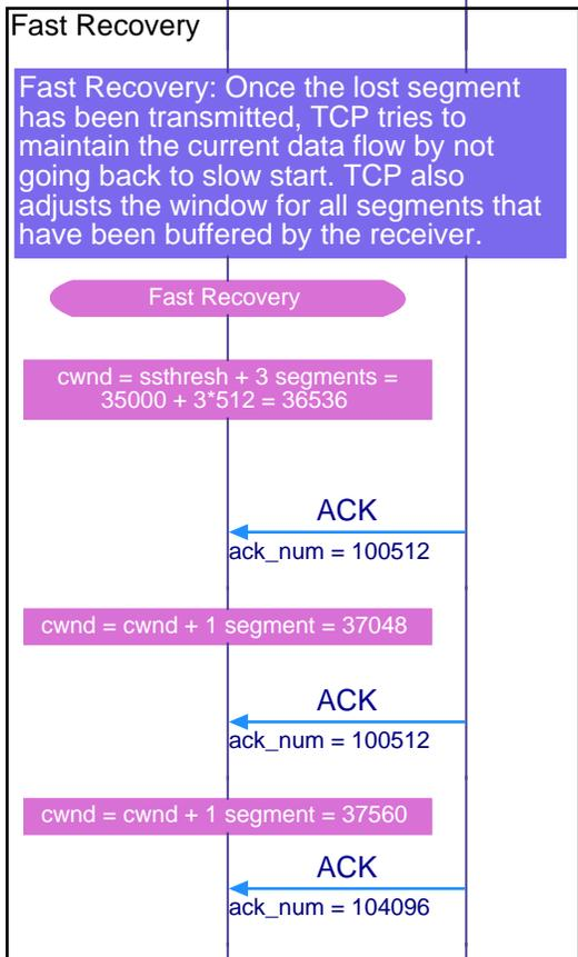
In "Fast Recovery" state, TCP's main objective is to maintain the current data stream data flow.
