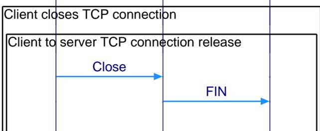
Client application wishes to release the TCP connection
